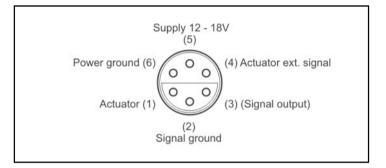
Fig. 5.2 LEMO socket output connections (external view)
