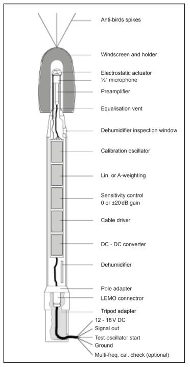
Fig. 2.1 Main components of the Outdoor Microphone System
