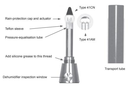
Fig. 2.4 Showing microphone assembly - note the difference between the two rain-protection caps
