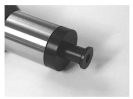
Fig. 3.4 1/4" microphone adapter inserted in the coupler
