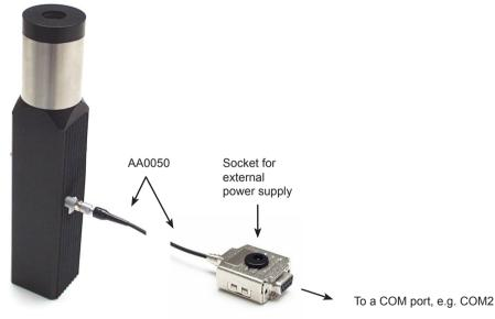
Fig. 4.1 Pistonphone connection to computer
