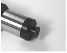
Fig. 3.5 <sup>1</sup>/<sub>8</sub>" microphone adapter inserted in the coupler
