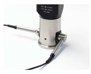
Fig. 5.1 Two-port Coupler RA0024 shown here with the two phase-matched microphones of an intensity probe
