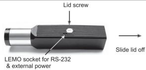
Fig. 3.1 Access to batteries
