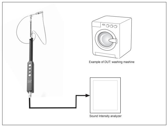
Fig. 5.1 Example of application setup: measuring the sound intensity of a washing mashine
