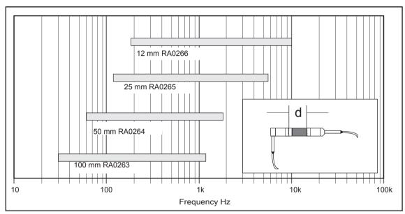
Fig. 2.6 Frequency ranges covered by the various spacer lengths.
