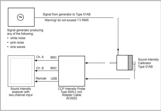
Fig. 4.3 Setup with signal generator and sound intensity analyzer
