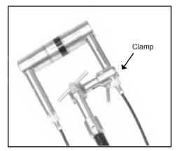
Fig. 3.5 Probe head mounted on the probe (straight setup)
