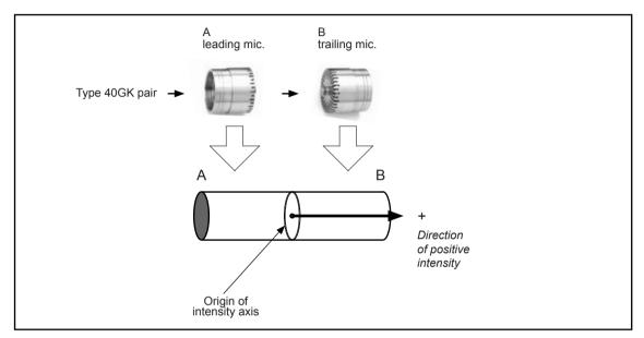
*Fig.* 5.2 Showing the microphones 'A' and 'B' which correspond with channels A and B respectively. 'A' is the leading microphone and is struck first by a sound wave
