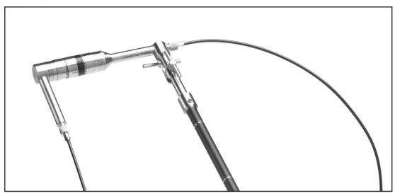
Fig. 3.1 Straight setup using the 25-mm spacer
