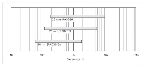
Fig. 4. Frequency ranges covered by the various spacer lengths.
