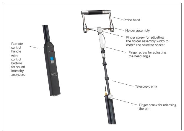
Fig. 1. The 50GI-RP Intensity probe.
