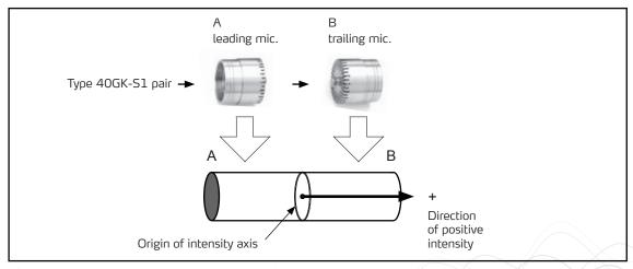
**Fig. 5.** Showing the microphones 'A' and 'B' which correspond with channels A and B respectively. 'A' is the leading microphone and is struck first by a sound wave
