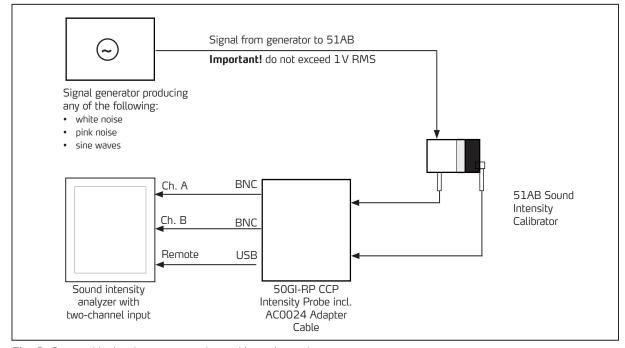
**Fig. 9.** Setup with signal generator and sound intensity analyzer.
