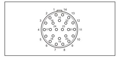
Fig. 4.1 External view of the pin numbers of the 24-pin LEMO female socket ECG.3B.324 at the base of the Type 50VI - 1 & 3 (see also Table. 4.1)
