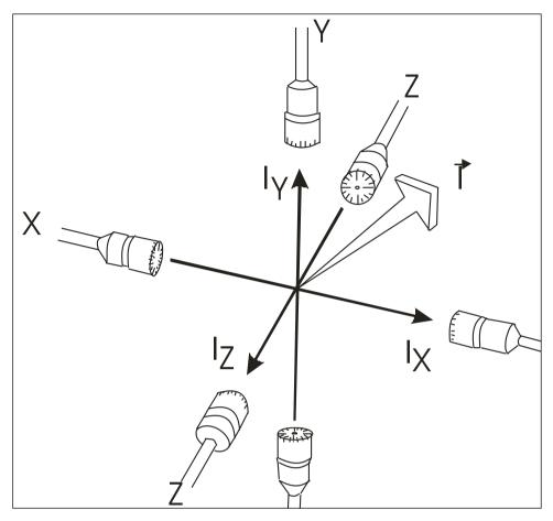
Fig. A.4 The three mutually orthogonal components  $(I_x, I_y \text{ and } I_z)$  of the resultant intensity vector **I**
