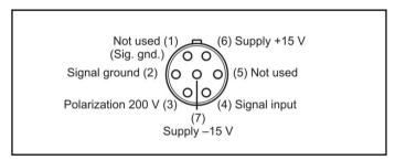
Fig. 4.1.1 7-pin LEMO female socket 1B (external view)
