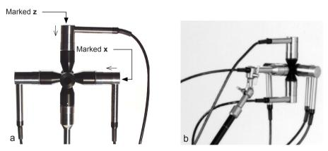
Fig. 5.4 Mounting the microphones of the X-axis (see Fig. 5.3b) and Y-axis (see Fig. 5.3c) on the spacer.
