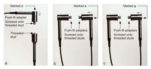
Fig. 5.1 Assembly of microphones, adapters and preamplifiers. Note: each picture shows a unique pair of phase-matched microphones Type 40AI. Do not mix up the pairs. A close up of a push-fit adapter is shown in Fig. 5.2.
