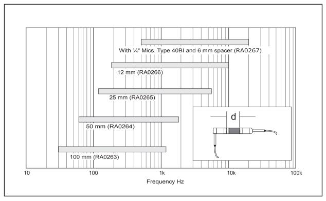
*Fig. 6.1* Working frequency ranges covered by the various spacer lengths. The top bar is for the case when a Type 50VX is equipped with a pair of 1/4-inch intensity microphones (Type 40BI) and a 6 mm spacer (note the extended high-frequency range)
