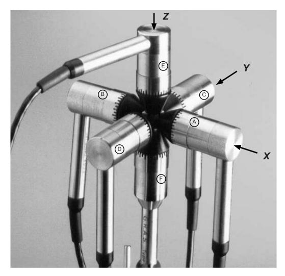
*Fig. 2.2* Showing the channels (A,B,C,D,E and F), and the positive directions of the X-Y-Z axes for each pair of probe microphones
