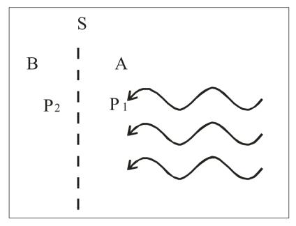
Fig. A.3 Transmission of power from system **A** to system **B** across an imaginary surface S
