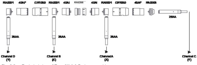
Fig. 5.5 Exploded view of Type 50VI-3 Probe assembly.
