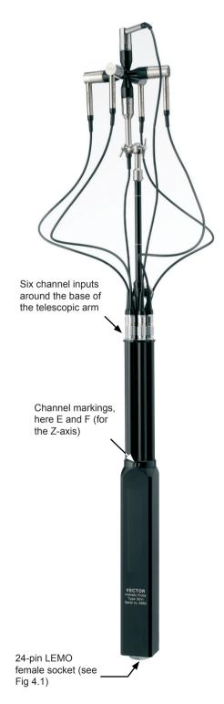
Fig. 2.1 Channel markings (here for the Z-axis) and the location of the 24pin LEMO socket
