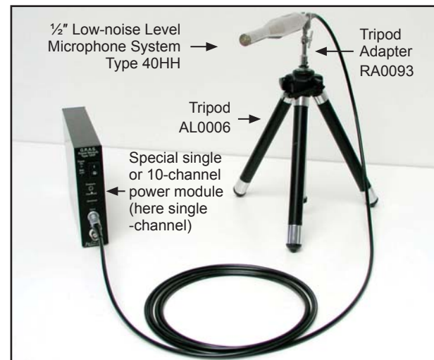
Fig. 2 A complete single-channel low-noise level measuring system
