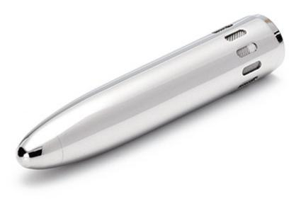
Length: 36.7 mm Outer diameter: 7.0 mm Threading (mic. protection grid threading): 6.35-60 UNS-2 Material: stainless steel Weight: 7 g The RA0022 is specially designed and optimized for use with 1/4" microphones for sound pressure measurements, when high speed wind comes from one known direction e.g. in a wind tunnel.
