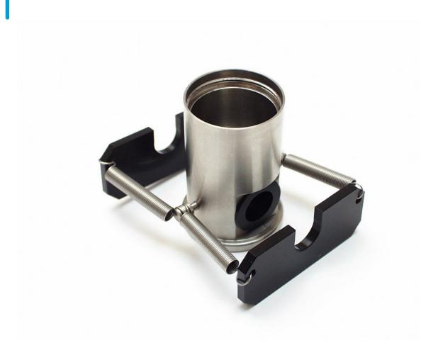
Two-port high-pressure coupler for 1/2" microphones. Used in comparison calibrations between two 1/2" microphones; one of which is a reference microphone. It can also be used in measuring the P-I (Pressure-Intensity) Index of intensity probes at 250 Hz. For use with GRAS 42AC Pistonphone.
