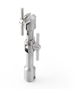
Material: Stainless steel Dimension: For 1/4" Special feature: Adjustable in 45 degree steps The GRAS RA0096 is an adapter for mounting a microphone set (microphone/preamplifier) on tripods having a standard 1/4" UNC-20 male thread. The adapter is provided with a clamp for attaching a 1/4" diameter preamplifier. The microphone can be set in angles between 0 and 180 degrees in 45 degree steps.
