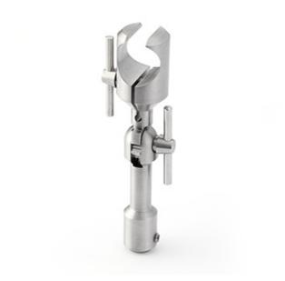
Material: Stainless steel Dimension: For 1/2" Special feature: Freely adjustable The GRAS RA0093-S1 is an adapter for mounting a microphone set (microphone/preamplifier) on tripods having a standard 1/4" UNC-20 male thread. The adapter is provided with a clamp for attaching at a 1/2" diameter preamplifier. The microphone can be set freely (stepless) in angles between 0 and 180 degrees.
