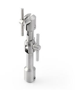
Material: Stainless steel Dimension: For 7 mm Special feature: Adjustable in 45 degree steps The GRAS RA0096-S1 is an adapter for mounting a microphone set (microphone/preamplifier) on tripods having a standard 1/4" UNC-20 male thread. The adapter is provided with a clamp for attaching a 7mm diameter preamplifier. The microphone can be set in angles between 0 and 180 degrees in 45 degree steps.
