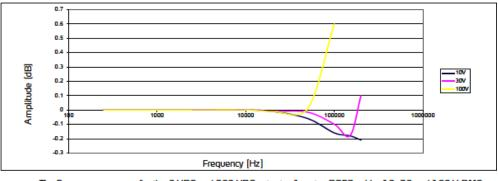
The Frequency response for the 0 VDC and 200 VDC outputs, 1 meter RG58 cable, 10, 30 and 100 V RMS.
