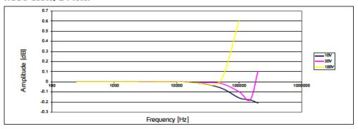
The Frequency response for the O VDC and 200 VDC outputs, 1 meter RG58 cable, 10, 30 and 100 V RMS.
