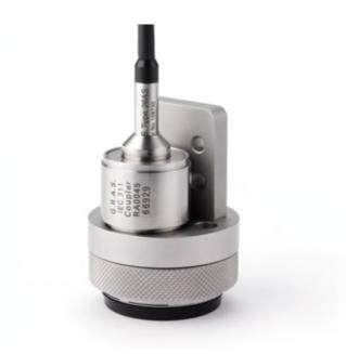
Connection: 0 V/CCP Volume: Complex Dyn range: 25 dB(A) to 150 dB ANSI: S3.7 IEC: 60318-1 & -2 This GRAS 43AH ear simulator with TEDS consists of the ITU-T Rec. P.57 Type 2 Ear Simulator and Type 3.2 Simplified Low-leak Pinna Simulator and is designed for making ITU-T standardized tests of telephone handsets, receivers and receiver/loudspeaker-modules on the production line.
