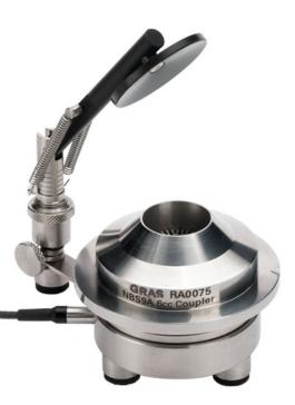
Connection: 200 V/LEMO Volume: 6 cc Dyn range: 14 dB(A) to 146 dB ANSI: S3.7 IEC: 60318-3 The GRAS 43AF-S1 Artificial Ear is a complete test jig for acoustically testing telephone handsets and earphones and complies with ANSI S 3.7 – 1995 – American National Standard for Testing Earphones.:
