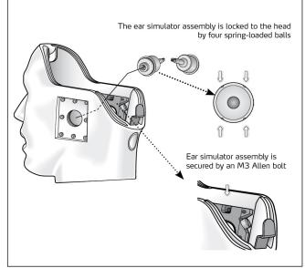
The transducers are mounted and removed by a simple snap fit mechanism.
