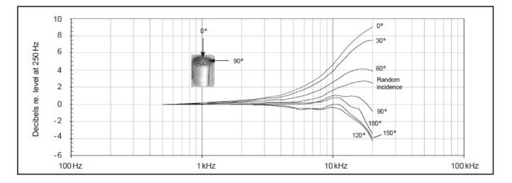
Free-field corrections for different angles of incidence
