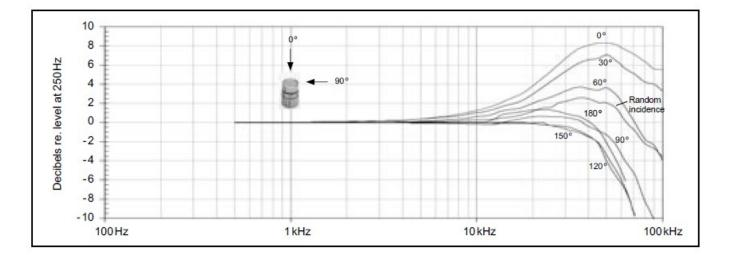
Free-field corrections for different angles of incidence
