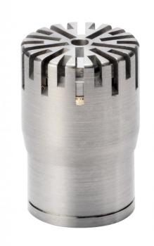
Freq range: 4 Hz to 80 kHz Dyn range: 30 dB(A) to 168 dB Sensitivity: 4 mV/Pa The 40BE is an IEC 61094 WS3F 1/4" prepolarized freefield microphone with rear-venting. The externally polarized equivalent is 40BF. **NOTE:** Optimized for use without protection grid—remove grid before measuring.
