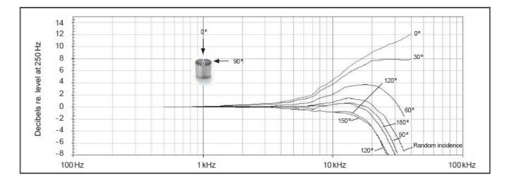
Free-field corrections for different angles of incidence
