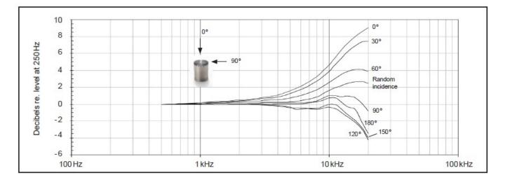
Free-field corrections for different angles of incidence
