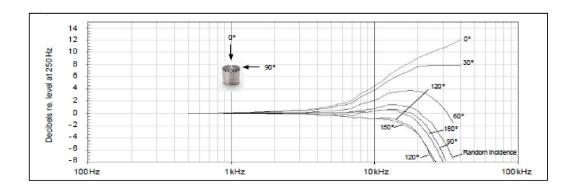
Free-field corrections for various degrees of incidence
