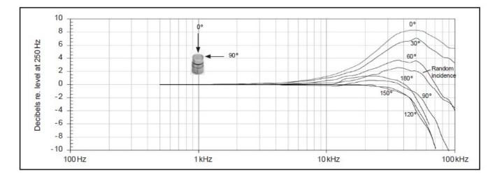
Free-field corrections for different angles of incidence
