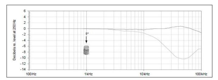
Typical frequency response (without protection grid). Upper curve shows free-feld response for 0°, lower curve shows pressure response.
