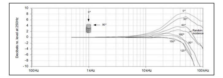
Free-field corrections for different angles of incidence
