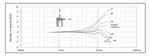
Free-field corrections for different angles of incidence
