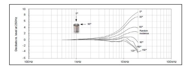
Free-field corrections for different angles of incidence
