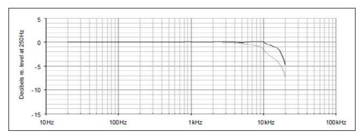
Typical frequency response. Upper curve shows response in a diffuse sound field (random incidence), lower curve shows pressure response.
