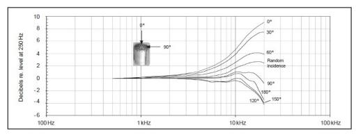
Free-field corrections for different angles of incidence
