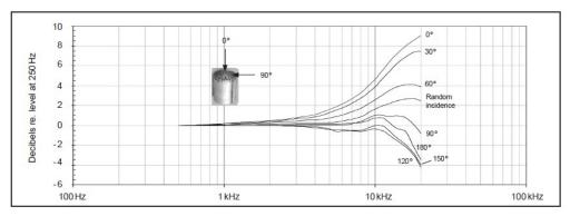
Free-field corrections for different angles of incidence
