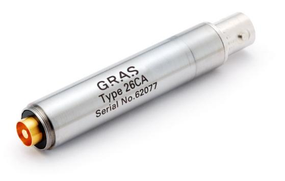
Freq range: 2.5 Hz - 200 kHz Noise: 1.8 µV Gain: -0.30 dB Special feature: General purpose The GRAS 1/2" Preamplifier GRAS 26CA is a general purpose preamplifier optimized for use with prepolarized condenser microphones. It is a small,robust unit and uses a GRAS CCP power supply (ICP ®), e.g. GRAS 12AL. It has a very low inherent noise level, and a large dynamic range and a frequency response from below 2 Hz to above 200 kHz.
