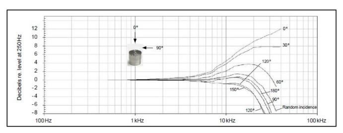
Free-field corrections for different angles of incidence
