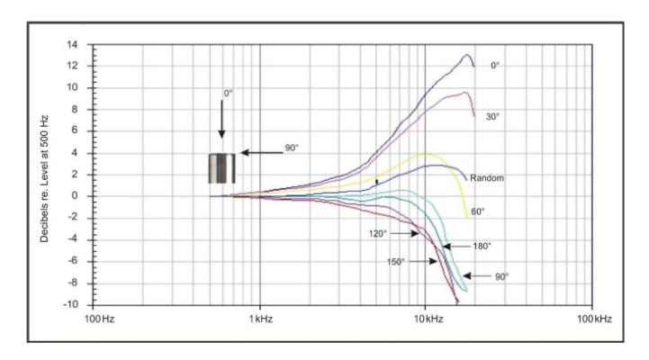
Free-field corrections for various angles of incidence
