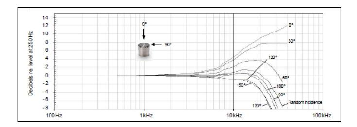
Free-field corrections for various degrees of incidence
