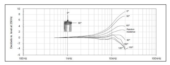
Free-field corrections for different angles of incidence
