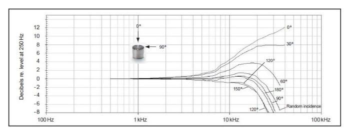
Free-field corrections for different angles of incidence
