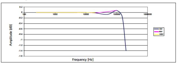
The Frequency response for the 0 VDC and 200 VDC outputs, 3 meter RG-58 cable, 10, 30 and 100 V RMS.
