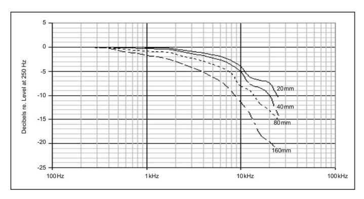
Frequency response for various lengths of stainless-steel probes
