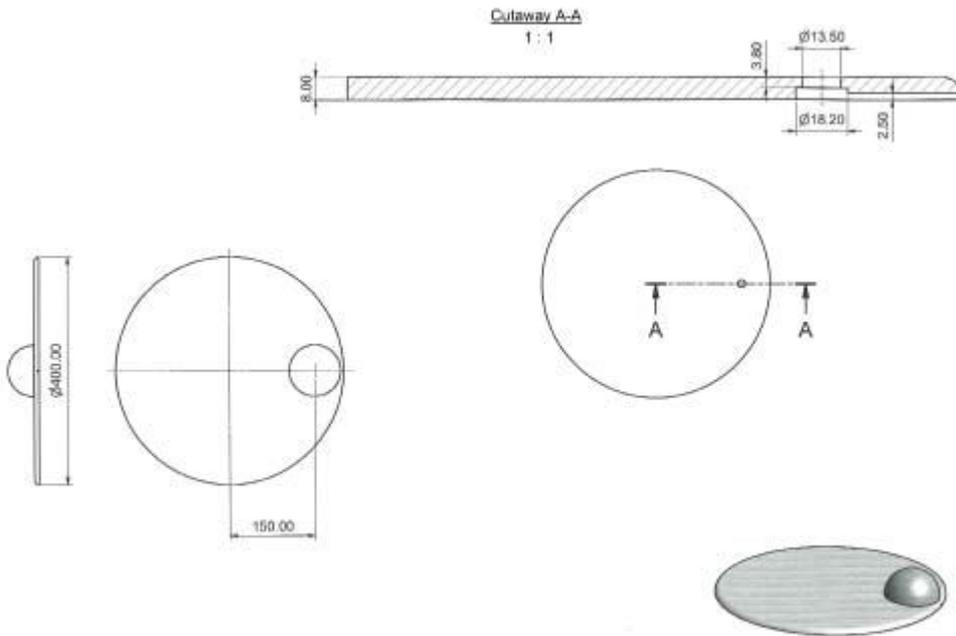
*Placement of the microphone in the plate with the windscreen on top. The cutaway of section A to A shows how the microphone fits into the plate.*
