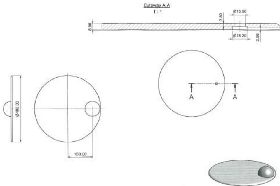
*Placement of the microphone in the plate with the windscreens on top. The cutaway of section A to A shows how the microphone fits into the plate.*
