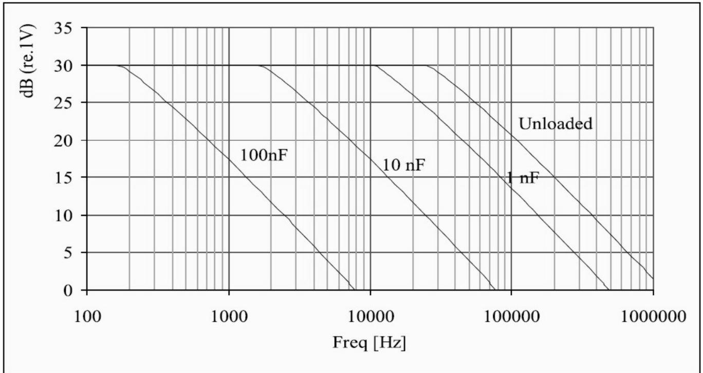
*Typical max. rms output signal with 120 V and 30 V supply*
