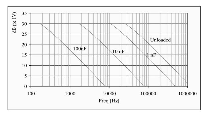
Typical max. rms output signal with 120 V and 30 V supply
