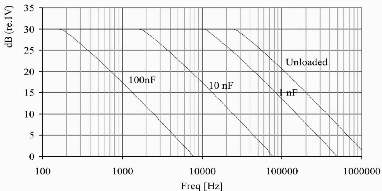
*Typical max. rms output signal with 120 V and 30 V supply*
