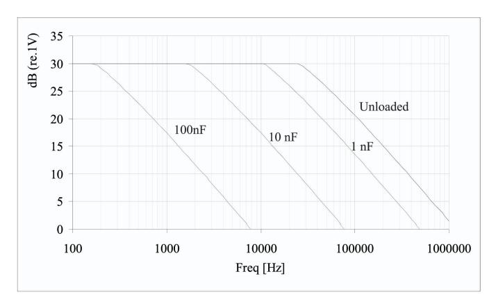
Max. RMS output signal for various cable loads with 120 V supply
