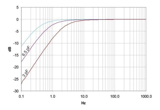
Typical low-frequency response of Type 26AL for ½ (20 pF), ¼ (6.5 pF) and ¼ (3 pF) microphones
