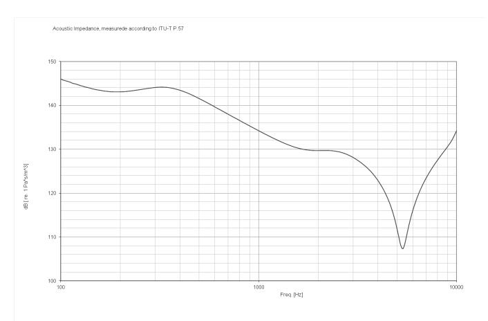
Acoustic input impedance of the RA0039
