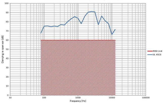
Self Insertion Loss, Measured with closed ear simulators: 100 Hz – 8 kHz >74 dB Self Insertion Loss, Measured with closed ear simulators: 80 Hz – 12.5 kHz >65 dB
