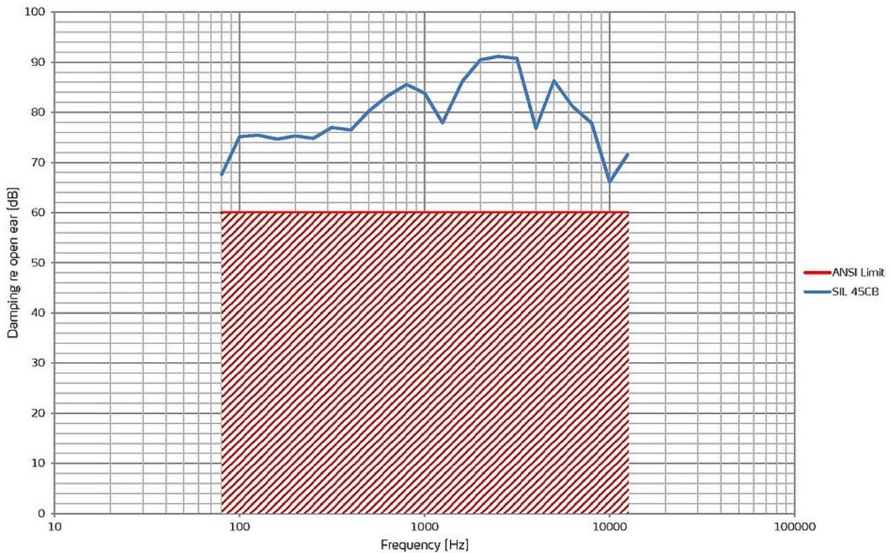
Self Insertion Loss, Measured with closed ear simulators: 100 Hz – 8 kHz >74 dB
