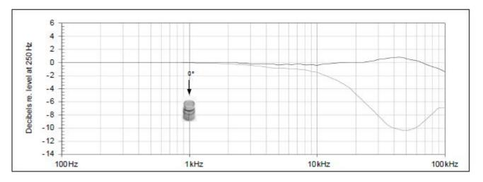
Typical frequency response (without protection grid). Upper curve shows free-field response for 0°, lower curve shows pressure response.
