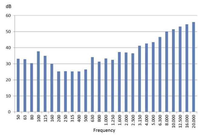
Self Insertion Loss measured in reverberant conditions
