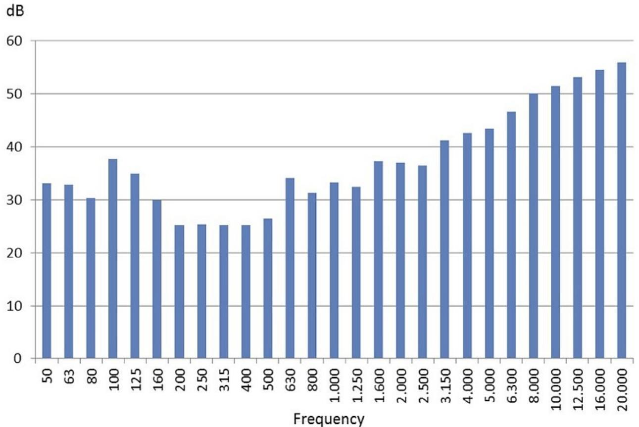
Self Insertion Loss measured in reverberant conditions
