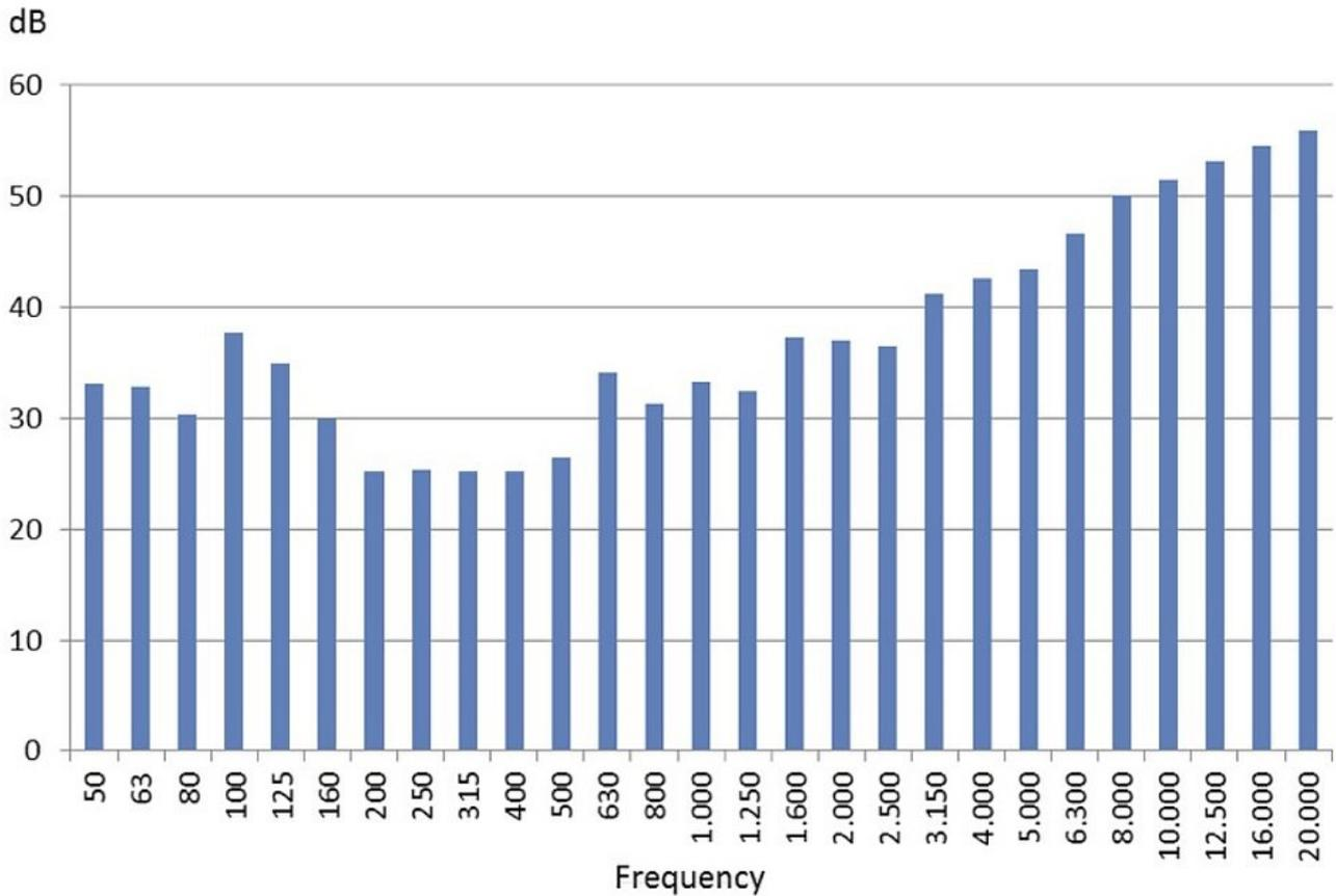
Self Insertion Loss measured in reverberant conditions
