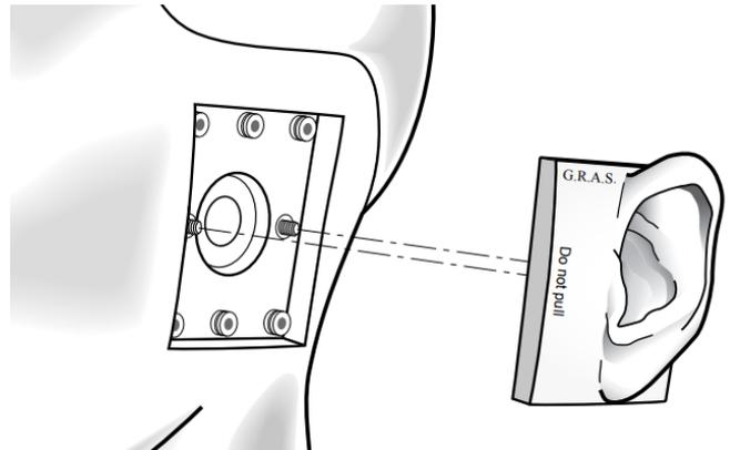
GRAS anthropometric pinna mounted on the 43AG test fixture's cheek plate using the RA0517 kit and finger screws (both included with the anthropometric pinna):
