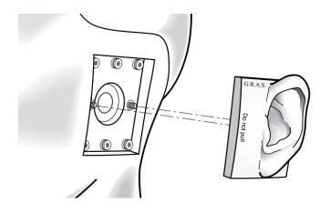
The external shape of the pinna is identical to that of the standardized KEMAR pinna, but concha and canal have been modified so that they closely mimic the properties of a real human ear. The ear canal has been extended and is an integral part of the pinna that now seals directly against the ear simulator. Like the human ear, the ear canal now has the 1st and 2nd bend, and the interface with the concha is oval.
