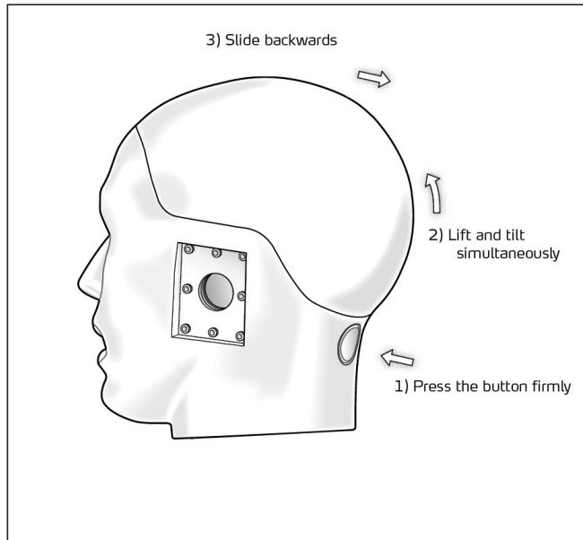
The interior of KEMAR's head can be accessed easily by pushing a button and lifting the scalp.
