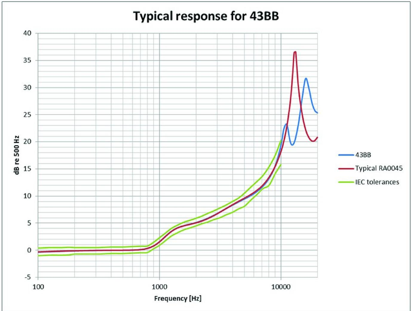
The frequency response is very similar to the standard 60318-4 ear simulator up to 10 kHz
