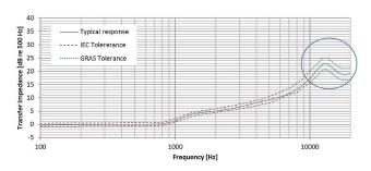
Fig 2. The half-wave resonance of a typical RA0402 High-Frequency Ear Simulator with IEC and GRAS tolerances
