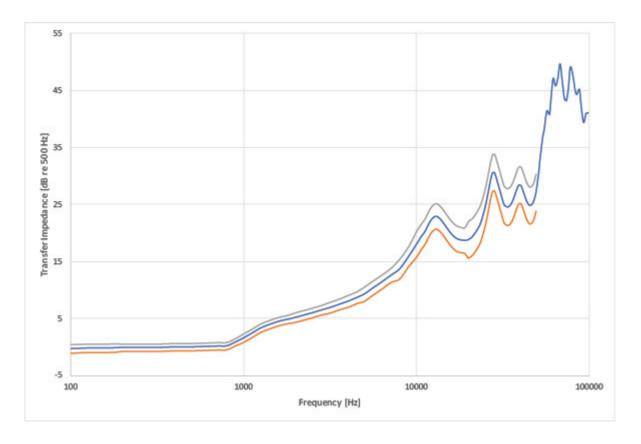
Fig 1. The transfer impedance of a typical RA0403 Hi-Res Ear Simulator with tolerances. Up to 10 kHz, the response is within the limits defined by IEC 60318-4. Above 10 kHz, the response is within a fairly tight tolerance band up to 50 kHz
