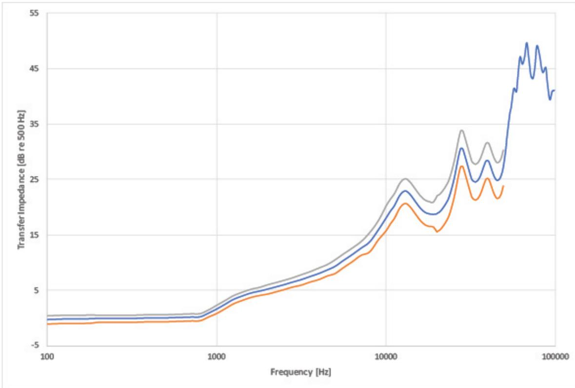
*Fig 1. The transfer impedance of a typical RA0403 Hi-Res Ear Simulator with tolerances. Up to 10 kHz, the response is within the limits defined by IEC 60318-4. Above 10 kHz, the response is within a fairly tight tolerance band up to 50 kHz*
