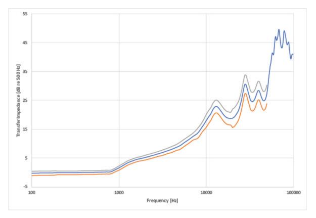
Fig 1. The transfer impedance of a typical RA0404 Hi-Res Ear Simulator with IEC and GRAS tolerances. Up to 10 kHz, the response is within the limits defined by IEC 60318-4. (red dotted curves). Above 10 kHz, the response is within a fairly tight tolerance band up to 50 kHz (green dotted lines).
